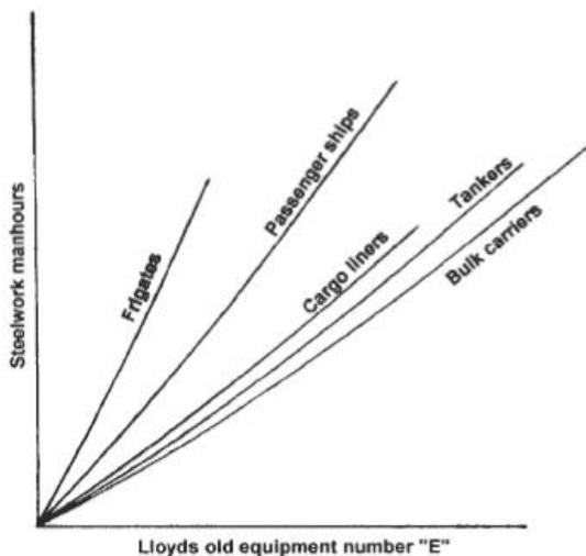
Fig. 4 Steelwork man-hours versus ship size.
