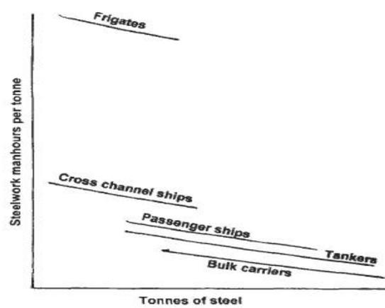
Fig. 3 Man-hours per ton versus steel weight.
