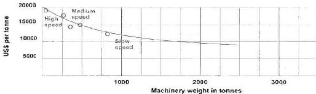
Fig. 11. Approximate costs of machinery per ton. Costs are on a 1993 basis and includee ude ma labor and overheads.
