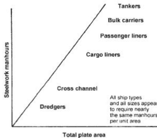
Fig. 5 Steelwork man-hours versus total plate area.
