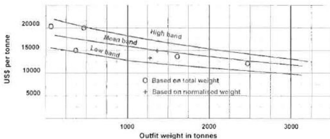
Fig. 10. Approx. costs of outfit per ton. Costs are on a 1993 basis include materials, labor and overheads.
