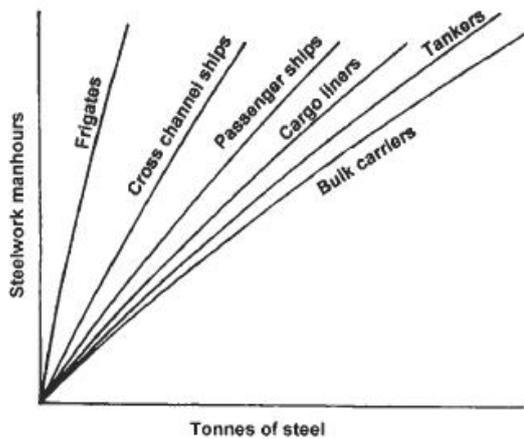
Fig. 2 Steelwork man-hours versus steel weight
