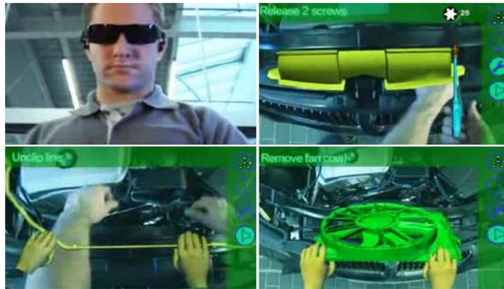
Fig.2 Augmented Reality in Maintenance and Repair [6].
