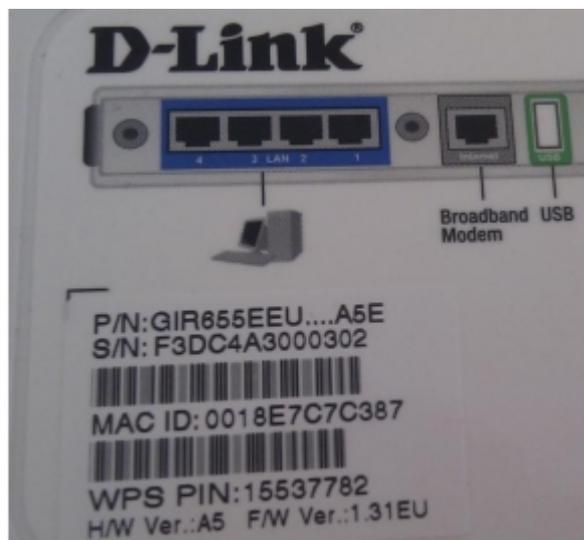
Label with WPS PIN on the back of a D-Link router
